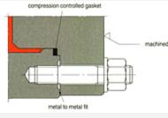
Pump flanges are full or spot faced on the back and designed for through-bolting.
