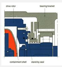
In case of leaking containment shell, the pressure inside the bearing bracket will increase and activate the seal. Leakage will be collected at the bottom of the bearing bracket and can be monitored by level detection device.
