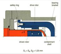
Due to the radial clearance  $S_2 > 1,25$  mm the pumps can handle non-metallic (non-ferrous) particles in the fluid up to 1,0 mm.
