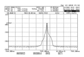
Typical 785nm SS Laser Spectrum
