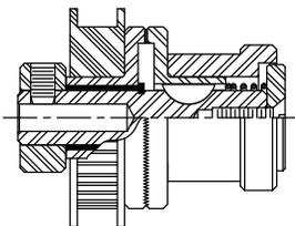
Phase adjustment shaft to pulley
