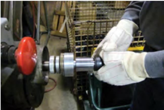
**Mechanical Safety** - The V-Series Slipper provides overload protection and increases operator safety to this manual cutting tool. This mechanical slip clutch limits the amount of torque that is transferred to the cutting tool, making this a safer operation for the user.
