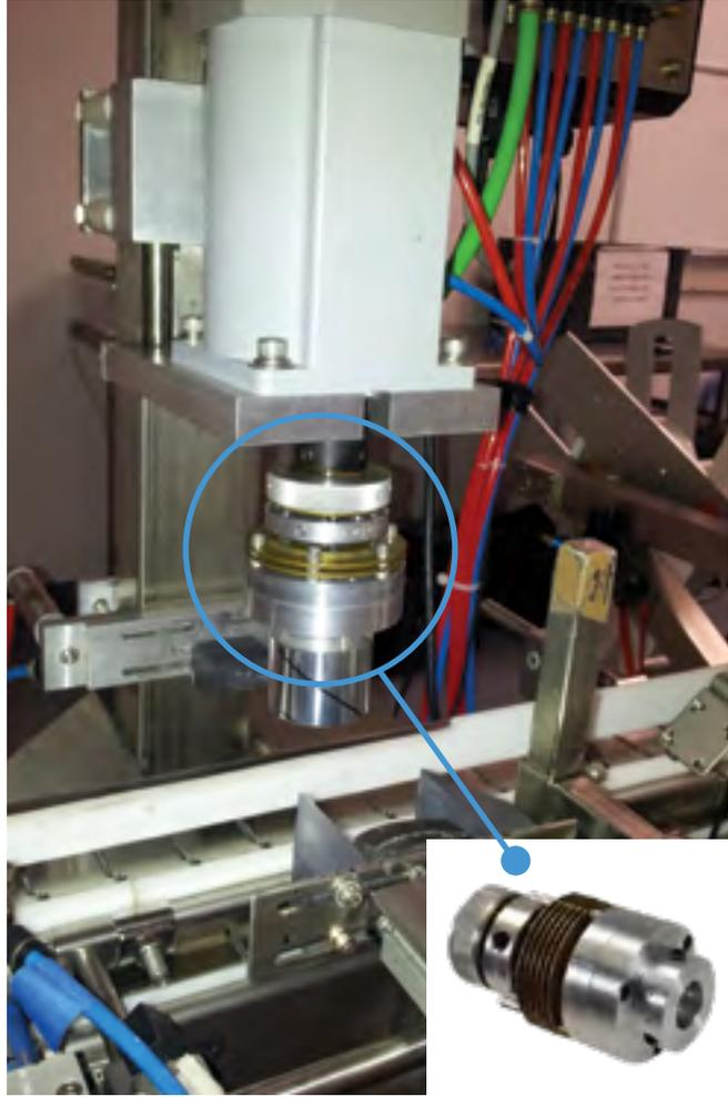
**Capping** - The V-Series slipper is the ideal solution for torque control on capping machines.
