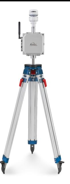
The **SENSIT® SPOD** is a highly advanced and innovative sensor system that is designed to detect VOC emission plumes and help locate the source of emissions. It is a low-cost and eco-friendly solution that uses wind and air pollutant concentration measurements to monitor the environment in real-time.
