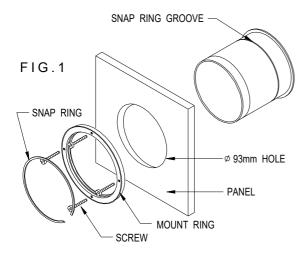
A panel mounting fastening kit is provided with all PLT Series Pressure Transmitter.
