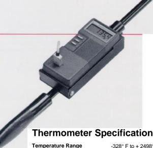
The Porta-Probe can operate for more than 1,200 hours continuously on a single 9-volt transistor radio battery. The 0.30" LCD display indicates temperature, scale in use (°F or °C), low battery and overranged or "open" sensor.
