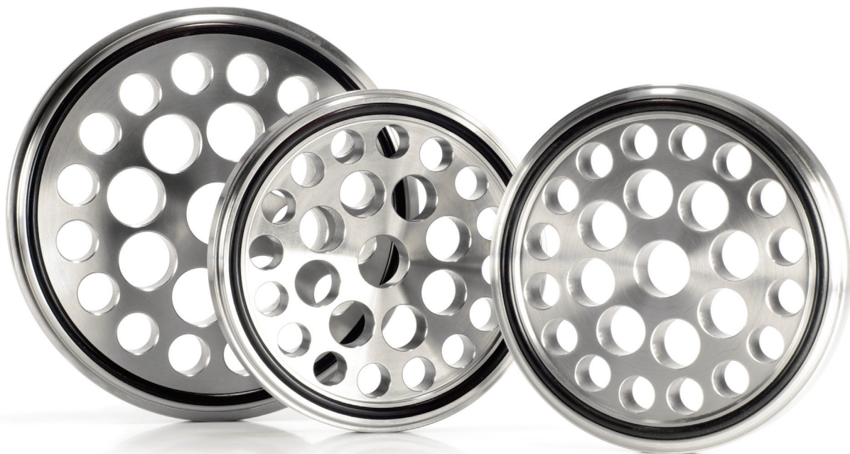
Canalta's Contour™ FCH Flow Conditioner Housing lineup utilizes a newly designed flow conditioning plate. These isolating flow conditioners incorporate a non-protruding HNBR seal around the downstream face to prevent bypass leakage and protect the integrity of the flow profile. Available in a variety of plate geometries, including Contour™ K5, Zanker, Spearman and others.
