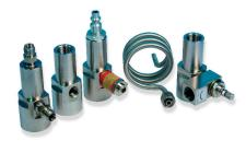
The sampling cells (from the left) DMT242SC2, DMT242SC and DSC74 can be used to connect the DM70 to sample gas flow. The DSC74B (right) is a two-pressure sampling cell that can be used for measurements in either pressurized or ambient pressure. The cooling/venting coil is included in the DSC74C sample cell, but is an option for all sampling cells.
