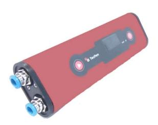
TecPen Fluid is a hand-held sensor system for determining the residual oxygen content in beverages such as beer, wine or soft drinks. It is attached directly to a sample outlet and rinsed with the beverage and measures thereby the residual oxygen content.
