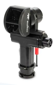
The scanning sonar head and integrated mechanical pan and tilt mechanism generates both sector scans and spherical scan data. The BV5000 MK2's 3D laserlike scanning capabilities and seamless integration with traditional laser scan imagery produce great results even in low and zero visibility conditions.
