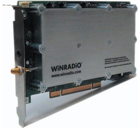
The WinRADIo WR-G305i is the first software-defined VHF/UHF scanning receiver on a PCI card.
