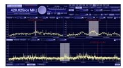
There are two concurrent DDC channels with 24 selectable output bandwidths ranging from 20 kHz to 4 MHz and the other from 20 kHz to 2 MHz.. Each can be used as an independent "virtual receiver". There is also a simultaneous 16 MHz wide real-time spectrum analyzer.
