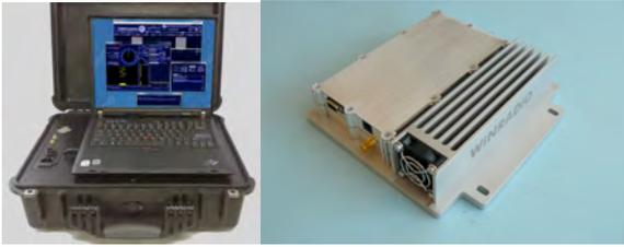
The receiver system is mounted within a portable enclosure and can be powered either from AC mains or from automotive DC employing optional converters. This allows for stationary and transportable deployment.
