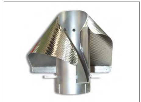
Fig.: forming collar for skewed fin seam, tight
