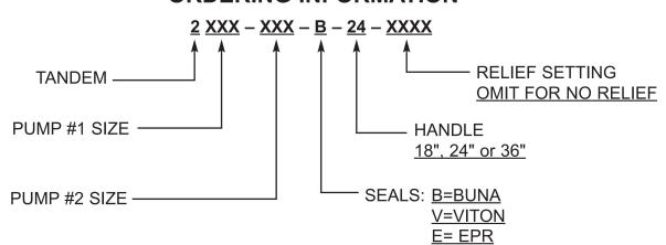
Standard sizes are 030 for 3/8, 040 for 1/2", 050 for 5/8", 060 for 3/4", 080 for 1", 120 for 1-1/2", 124 –125-126 are for two stage configurations. Any two size pumps can be combined, maximum pressure rating is a function of the final configuration, consult engineering for rating. When operated together the displacements and handle forces are cumulative, add for total displacement and force.
