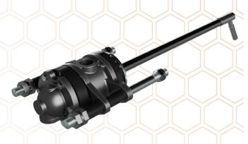
The SlimLine elbow syphon maintains its position at higher rotational speeds, enabling maximum condensate removal in high-speed corrugators. Utilizing a tapered wedge, heavy-duty retention nut, and custom-engineered locking key, the SlimLine elbow syphon integrates seamlessly to the SecureLock™ retention plate inside the LJX-PT rotary joint, maintaining proper syphon clearance.
