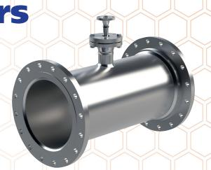
Kadant desuperheaters are custom designed for each application and are available in various materials. The simple yet efficient designs allow for direct installation into the steam pipeline with flanged connections. All desuperheaters can be installed in either horizontal, vertical, or diagonal pipelines providing there is sufficient straight run both upstream and downstream of the desuperheater.
