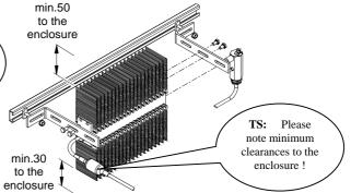
The brackets in zinc coated steel and fixing bolts illustrated above are included with the heater. Furthermore, a short threaded rod for mounting the TAE thermostat on the heater is supplied with the TAE.
