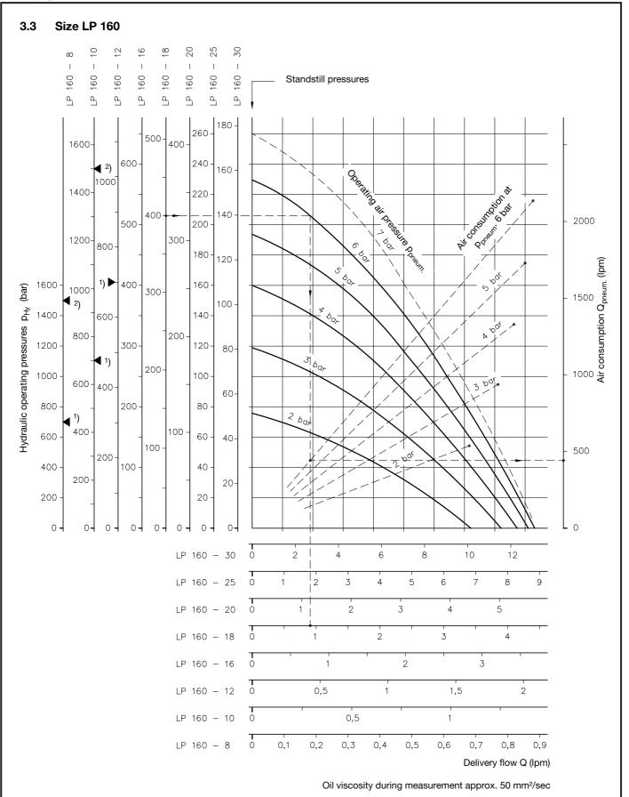
Example: A pump type LP 160-18 delivers a flow of approx. 0.9 lpm at a pneum. pressure of 6 bar and a hydr. pressure of 400 bar. Air consumption will be approx. 500 lpm. The standstill air pressure is approx. 5.3 bar (pneumatic pressure, where the pump starts up against a hydraulic pressure of 400 bar).
