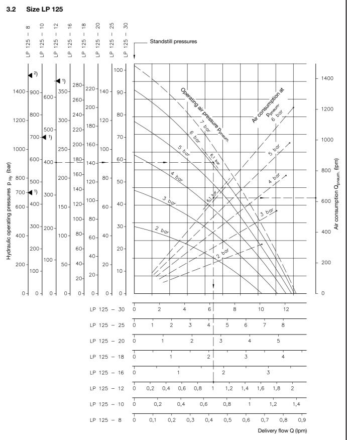
Oil viscosity during measurement approx. 50 mm²/sec
