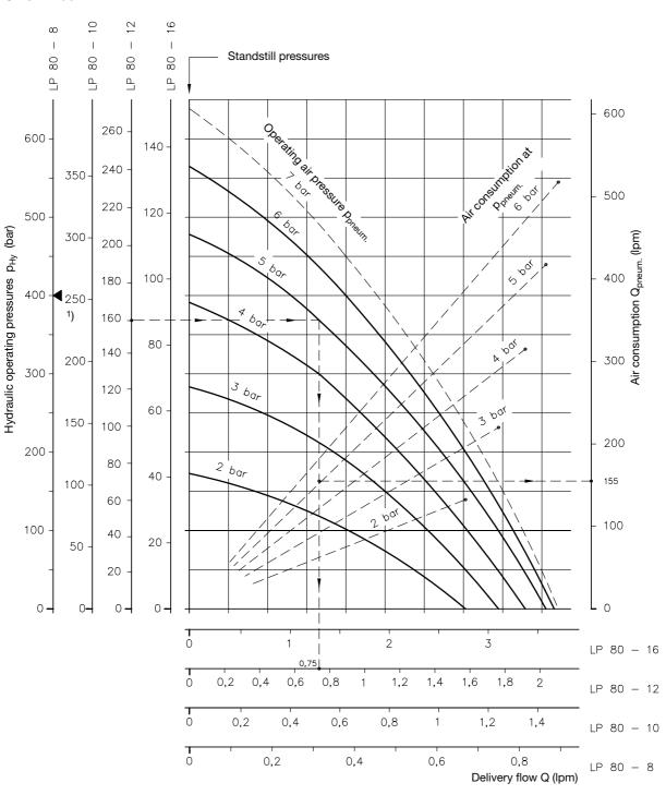
Oil viscosity during measurement approx. 50 mm²/sec
