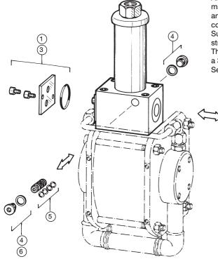
Any industrial standard hydraulic oil (ISO VG 10) or spindle oil (ISO VG 5 to 10) may be used in the pneumatic maintenance unit. The dynamic seals of piloting and main plunger of the reversal control valve should be lubed regularily when connected to oil-free pneumatics and a frequent all-day use is intended. Suited are longterm lubes e.g. Autol TOP 2000 from Co. Autol, Paradies-straße 14, D-97080 Würzburg.
