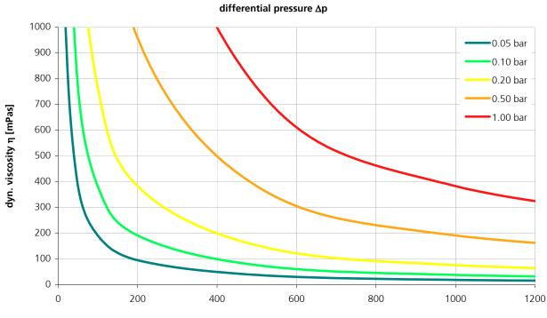
volumetric flow Q [ml/min]
