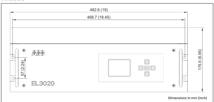
Note: Only the front view of the housing (with its height differing from the standard dimension) is depicted in this dimensional drawing. Refer to the dimensional drawing on page 36 for other views and dimensions of the 19-inch housing.
